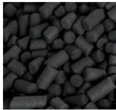
AdFis siloxane removal Activated carbon
